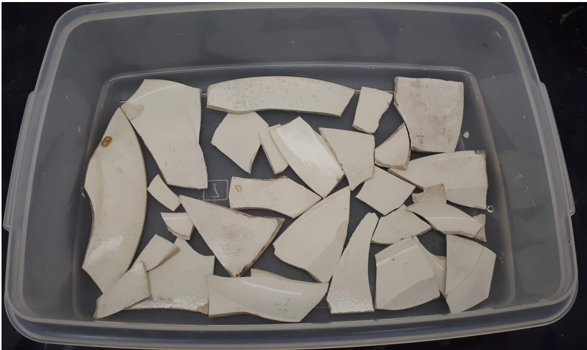
Figure 8 : RO water rinse, following 3% hydrogen peroxide soak.
